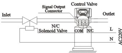
Figure 3-3 Wiring of Solenoid Valve on Inlet
