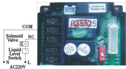
Figure 3-2 Wring of Solenoid Valve on Outlet
