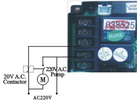
Figure 3-9 Wiring of Booster Pump on Inlet
