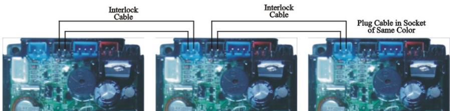
Figure 3-10 Network System Wiring with Interlock Cable
