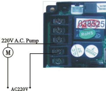
Figure 3-8 Wiring of Booster Pump on Inlet
